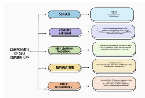
A **flowchart** illustrating a self-driving car's algorithm typically consists of blocks and arrows representing the vehicle's responses to its environment. The core components include:
